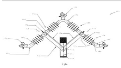
Insulator integrated framings for power lines and kits for assembling same are disclosed. The framings have retaining member assemblies configured to retain power line wires and conductors, separated from power line support structures and other retaining member assemblies by insulators.
